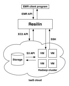
The client program will interact with the service through EMR requests. Resilin receives the client requests and translates them in two types of actions: EC2 requests to the IaaS cloud for starting or terminating instances and remote connections using SSH protocol to the instances for Hadoop configurations.
