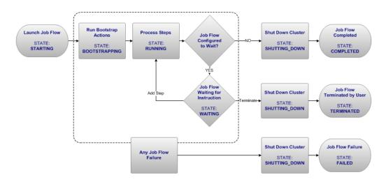
The jobflow is in STARTING state from the creation until the cluster's instances are up and running. Then the EMR will run the bootstrap actions on each cluster node, setting the jobflow's state to BOOTSTRAPPING. When bootstrapping phase is done, the cluster is ready to run the MapReduce applications thus the jobflow goes to RUNNING state. All the jobflow's steps are executed sequentially during this phase.
