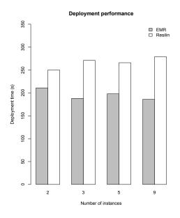
Both Amazon EMR and Resilin have a stable deployment time. The measurements show that Resilin is constantly slower than Amazon. As the Amazon EC2 architecture is not public, we don't know how they are propragating the virtual machine image or if they keep it in a cache on the hipervisor nodes.
